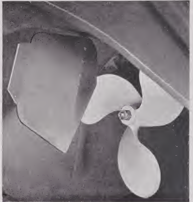
FIGURE 16. Revised rudder design with cutaway leading edge, rear tab, and sloping rudder post.
